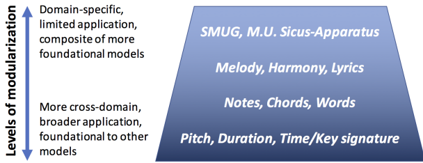
Figure 1: The pyramid shows examples of concepts at different levels of modularization. The highest level modules represent full-functioning MUME systems (e.g., SMUG (Scirea et al. 2015) and M.U. Sicus-Apparatus (Toivanen et al. 2013)) which are composed of lower level modules and have more narrow applications. Lower level modules represent subconcepts that are more broadly applicable and are foundational to more complex concepts. A modular approach to building MUME systems focuses on developing (potentially reusable) models at multiple levels.
